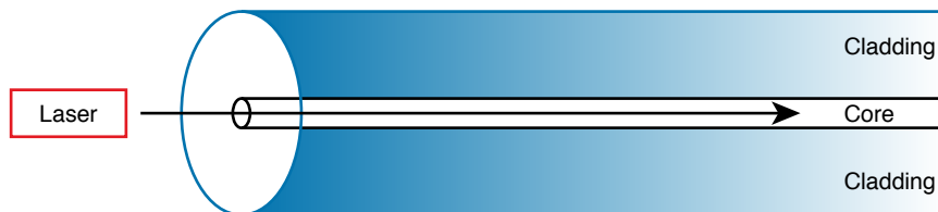
Figure 2-17 Transmission on Single-Mode Fiber with Laser Transmitter
