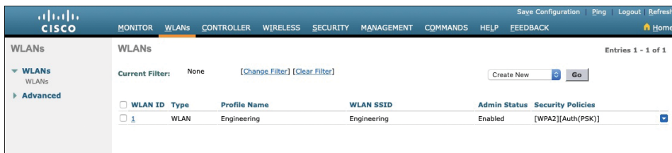
Figure 29-20 Displaying WLANs Configured on a Controller
