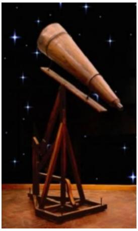
The purpose of the mount is to support the telescope, with minimum vibration, yet permit it to be readily pointed at a target and to track the target's movements. And, of course, if the telescope is not in an observatory, the mount has to be light enough so the telescope is still portable. These goals are not easily reconciled.
