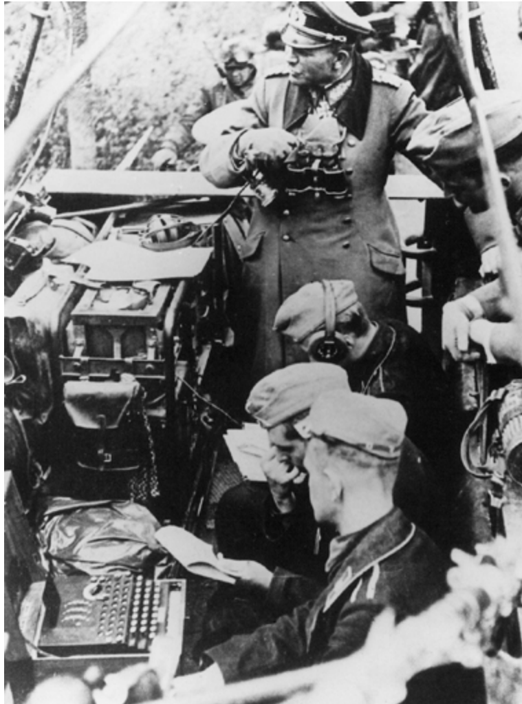
Figure 43 General Heinz Guderian's command post vehicle. An Enigma machine can be seen in use in the bottom left. ( photo credit 4.2 )
