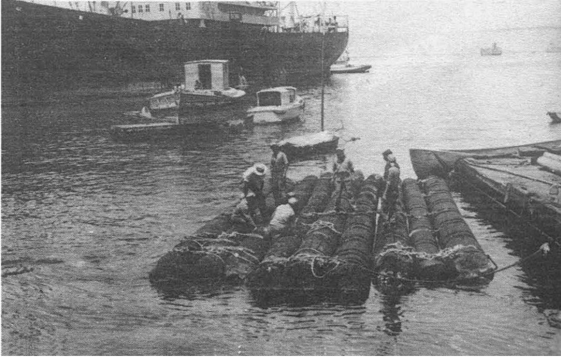
Building the raft in Peru. We lashed the nine big balsa logs to qether with ordinary hemp ropes, using neither nails nor metal in any form.
