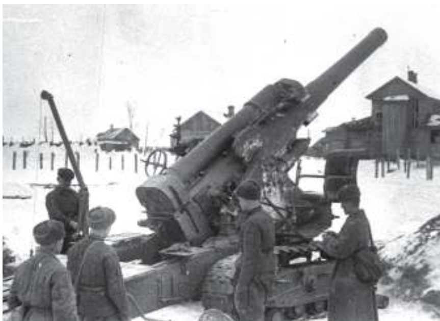
Soviet heavy artillery: a 280mm Br-5 M1939 mortar prepares to fire. (From the fonds of the RGAKFD in Krasnogorsk via Stavka)
