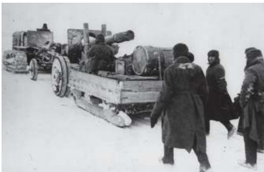
A 152mm ML-20, M1937 howitzer is moved into position by a Stalinets S-65 tractor with spare fuel and munitions on a sledge. (Nik Cornish at www.Stavka.org.uk )
