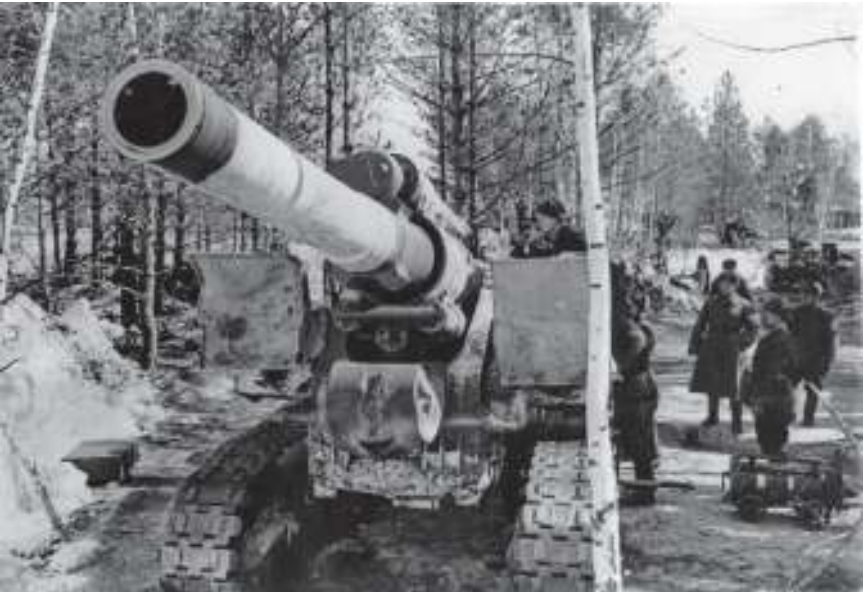
A tracked 203mm B-4, M1931 howitzer takes aim. (Nik Cornish at www.Stavka.org.uk )
