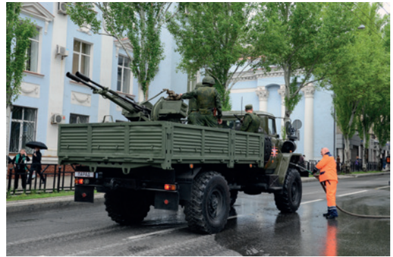
The militias on both sides have pressed a variety of improvised vehicles into service, such as this DNR gun-truck mounting a double-barrel ZU-23 cannon. Originally developed for short-range AA defense, the 23mm ZU-23 has found a second effective role as a direct-fire ground weapon. (Andrew Butko/Wikimedia Commons/CC-BY-SA 3.0)
