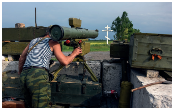
A rebel soldier in a position near Dokuchayevsk, 2015, mans a 9K111 Fagot wire-guided antitank missile, known in the West as the AT-4 Spigot. Dating from 1970, the AT-4 is typical of the kind of second-rank equipment that the rebels could either loot from government arsenals or receive as hand-me-downs from the Russians. Nonetheless, against anything but the most modern armor it was a serious threat. (Mstyslav Chernov/Wikimedia Commons/CC-BY-SA 4.0)
