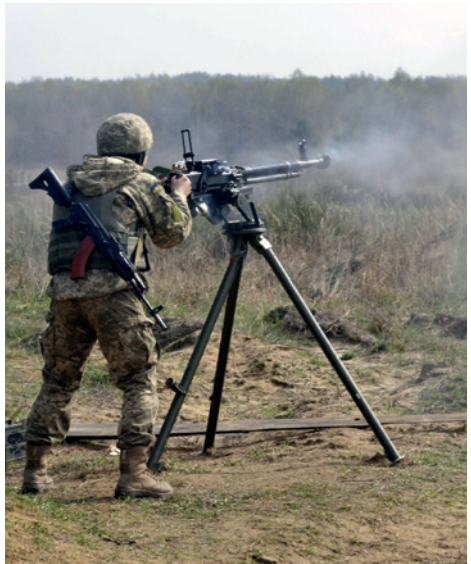
A Ukrainian government soldier in a particularly exposed position, firing a DShKM 12.7mm (.50cal) heavy machine gun. This modernized version of a design dating back to 1946 is still a brutally powerful weapon, if often inaccurate. (Public Domain/Staff Sgt Adriana M. Diaz-Brown)
