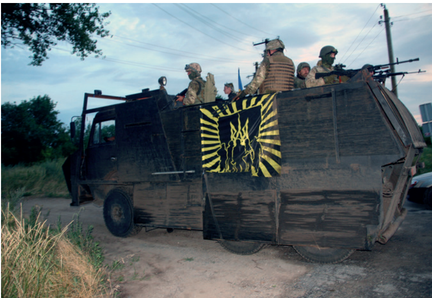
Militiamen from the Ukrainian Azov Bn advance in an open-topped truck with improvised armor. Such makeshift personnel carriers were relatively commonplace in the early stages of the war, but proved vulnerable even to modern rifles, let alone the ubiquitous rocket and grenade launchers, and have since been replaced with military vehicles. The symbol on the side is that of the Ukrainian Patriot movement. (Carl Ridderstråle/Wikimedia Commons/CC-BY-SA 4.0)
