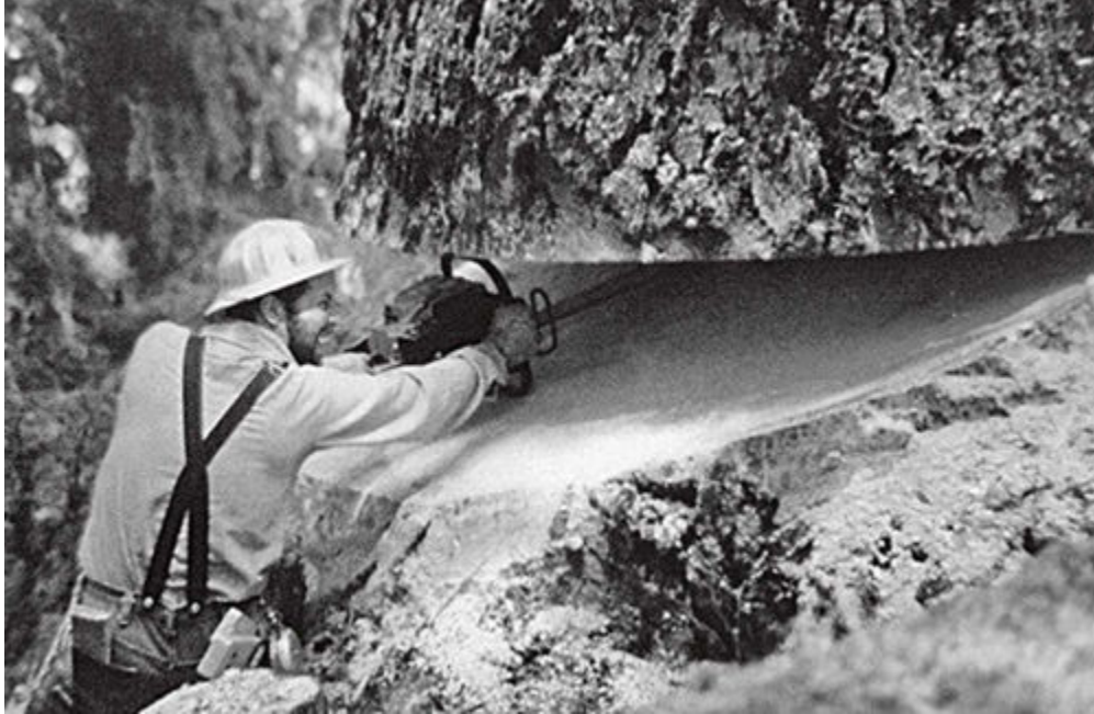
Felling a four-hundred-year-old Douglas fir, 8 feet in diameter across the stump and 260 feet tall. Photo from Jonsered's 1985 catalog for the American market. The saw is a Jonsered 920 Super.
