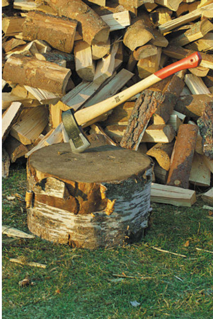
A low chopping block will give high speed and good impact to the blow. Here, a chopping block just 30 centimeters (12 inches) high is used with an Øyo ax.
