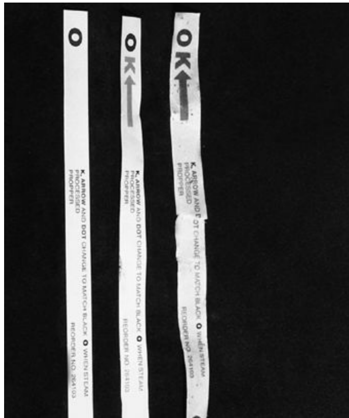
Heat-sensitive sterilization indicator strips showing no sterilization, partial sterilization, and complete sterilization.
