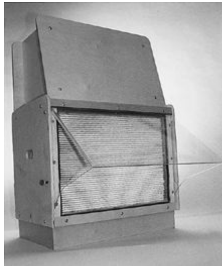
A laminar flow bench suitable for home or small-scale commercial cultivation.
