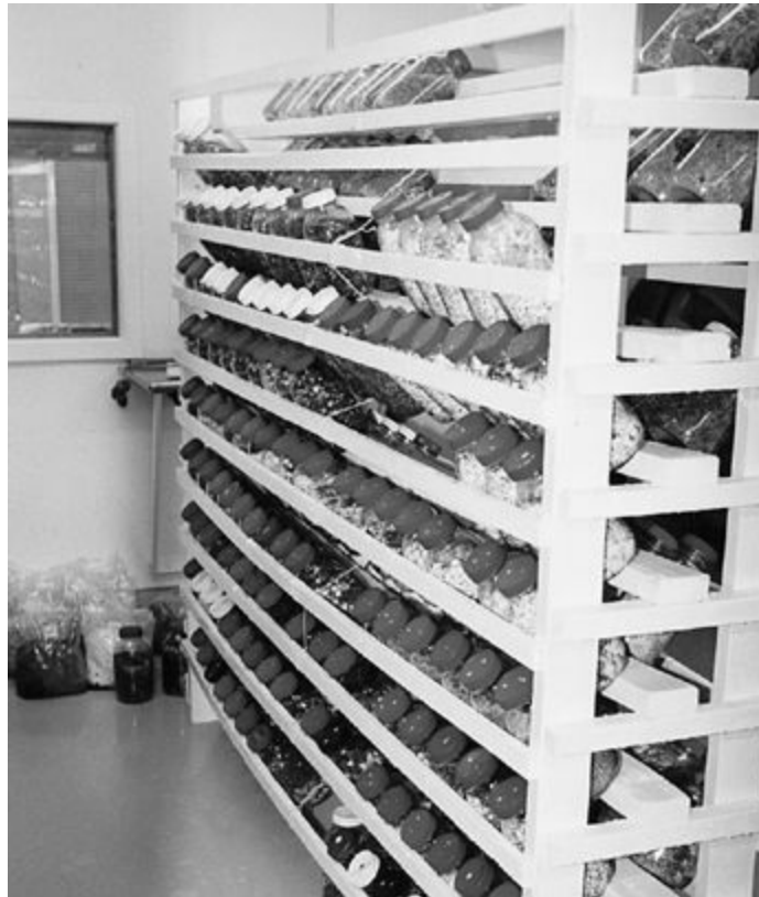
A space-efficient rack for incubating grain spawn in jars. Three hundred forty ½-gallon jars can be stored on this 8-foot long x 8-foot high x 16-inch wide shelf system. Spawn quality is improved by storing the jars at an angle. Earthquake sensitive.
