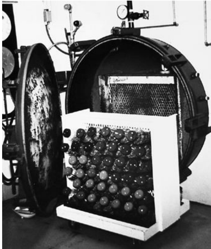
Grain-filled \frac{1}{2} -gallon jars ready for loading into a commercial autoclave.
