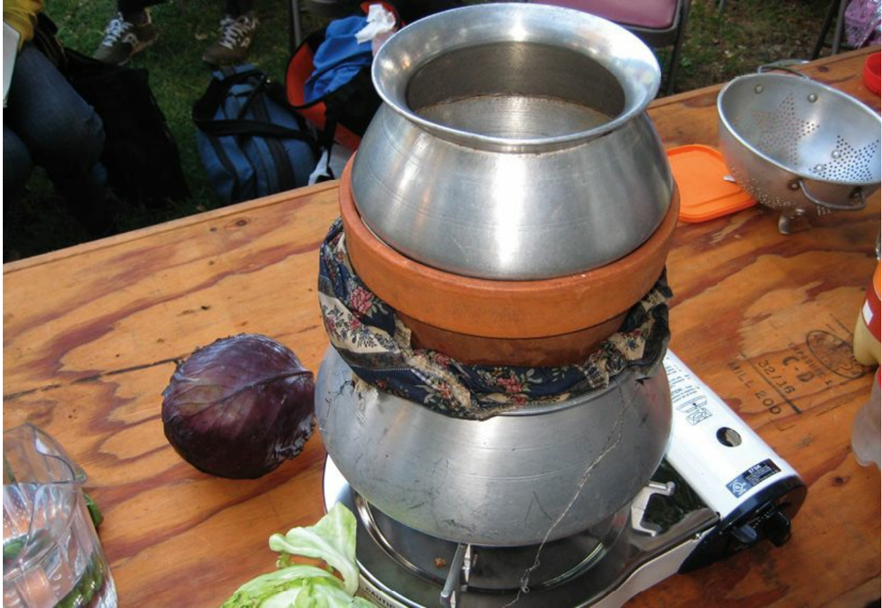
An improvised still constructed by Bhutanese and Nepali immigrants in Oakland, California, to make raksi .
