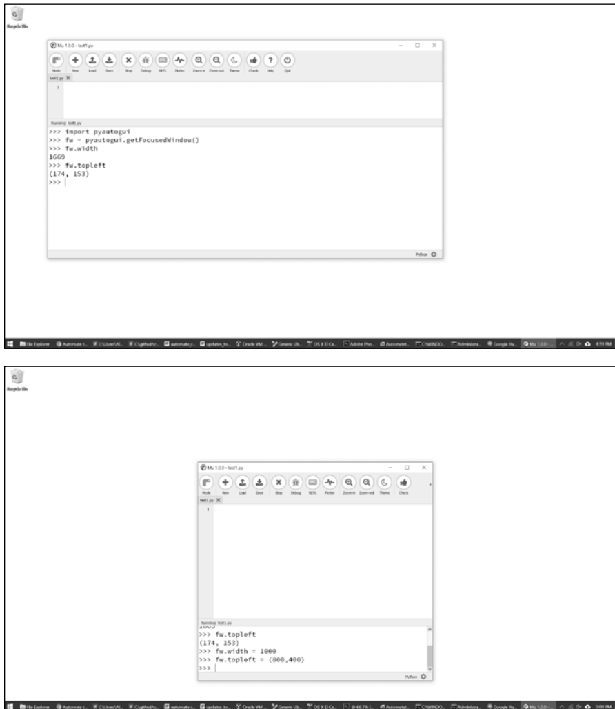
Figure 20-5: The Mu Editor window before (top) and after (bottom) using the Window object attributes to move and resize it
