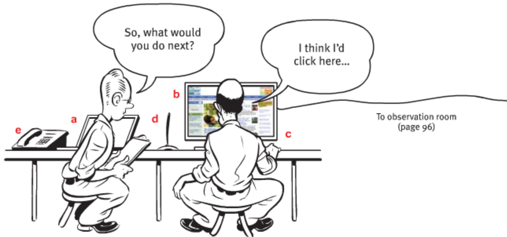
a Computer b External monitor and keyboard c Mouse d Microphone e Speakerphone
