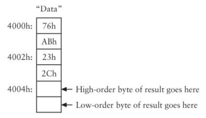
These six locations don't have to be all together like this. They can be scattered anywhere throughout the whole 64-KB Data RAM array. To add these values at these memory locations, you must set up the instructions in the Code RAM array, like this:
