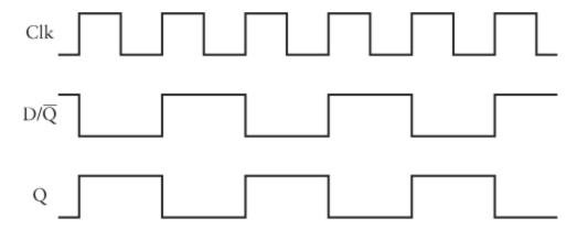
When the Clock input goes from 0 to 1, the value of D (which is the same as  $\overline{\mathbb{Q}}$ ) is transferred to Q, thus also changing  $\overline{\mathbb{Q}}$  and D for the next transition of the Clock input from 0 to 1.
