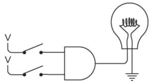
Notice that this symbol for the AND gate not only takes the place of two relays wired in series, but it also implies that the top relay is connected to a
