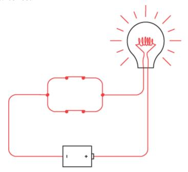
The lightbulb lights if the top switch *or* the bottom switch is closed. The key word here is *or*.
