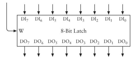
Or to be more consistent with the 1-bit latch, it can be drawn this way:
