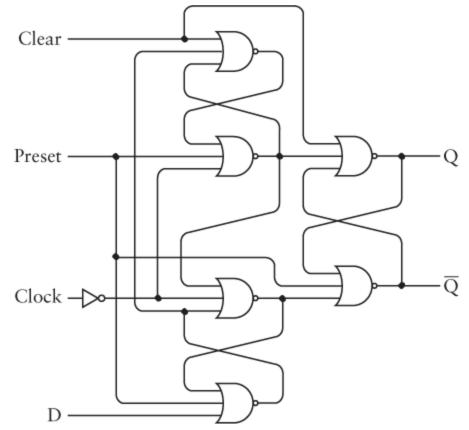
The Preset and Clear inputs override the Clock and Data inputs. Normally these two inputs are 0. When the Preset input is 1, Q becomes 1 and  $\overline{\mathbb{Q}}$  becomes 0. When the Clear input is 1, Q becomes 0 and  $\overline{\mathbb{Q}}$  becomes 1. (Like the Set and Reset inputs of an R-S flip-flop, Preset and Clear shouldn't be 1 at the same time.) Otherwise, this behaves like a normal edge-triggered D-type flip-flop:
