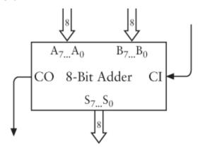
Normally (ignoring what we did with subtraction in the last chapter), the eight A inputs and eight B inputs are connected to switches, the CI (Carry In) input is connected to ground, and the eight S (Sum) outputs and CO (Carry Out) are connected to lightbulbs.
