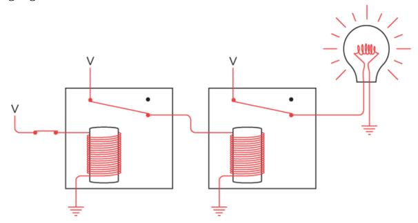
Connecting relays is the key to building logic gates.
