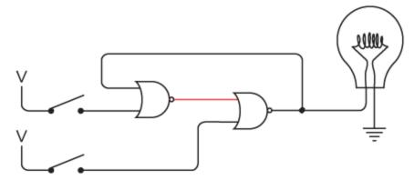
We're back where we started. At this time, you can close and open the bottom switch with no further effect on the lightbulb. In summary
