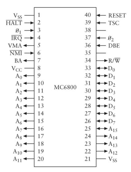
The  $V_{SS}$  indicates Ground, and  $V_{CC}$  is 5 volts. Like the 8080, the 6800 has 16 output Address signals and 8 Data signals used for both input and
