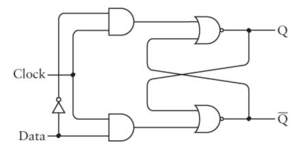
When the Clock input is 1, the Q output is the same as the Data input. But when the Clock input goes to 0, the Q output holds the last value of the Data input. Further changes to the Data input don't affect the outputs until the Clock input goes to 1 again. The logic table of the flip-flop is the following:
