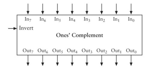
The Ones' Complement box, the 8-Bit Adder box, and a final exclusive OR gate can now be wired together like this:
