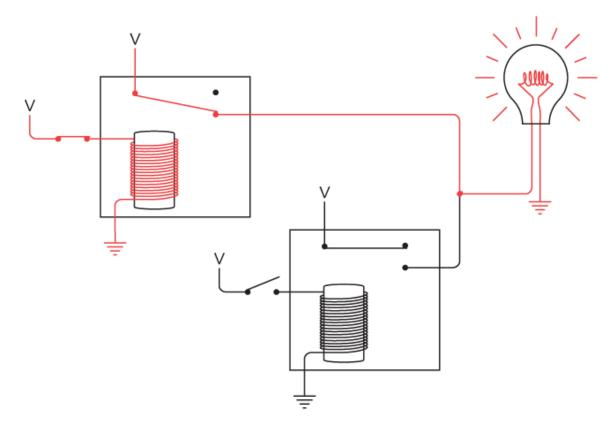
Similarly, if we leave the top switch open but close the bottom switch, the bulb lights up:
