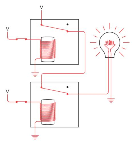
Now both relays are triggered, and current can flow between V, the lightbulb, and ground.
