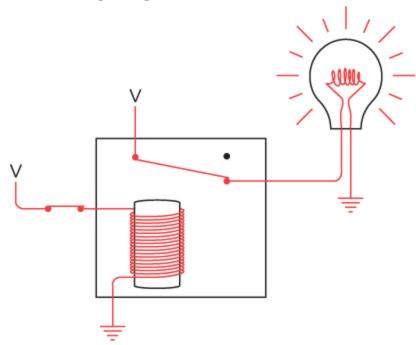
These diagrams of the relay show two voltage sources and two grounds, but in all the diagrams in this chapter, all the V's can be connected to one another and all the grounds can be connected to one another. All the networks of relays and logic gates in this chapter and the next will require
