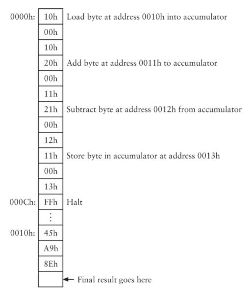
As usual, the instructions begin at 0000h because that's where the counter starts accessing the RAM array after it has been reset. The final *Halt* instruction is stored at address 000Ch. We could have stored the three numbers and the results anywhere in the RAM array (except in the first 13 bytes, of course, because those memory locations are occupied by instructions), but we chose to store the data starting at address 0010h.
