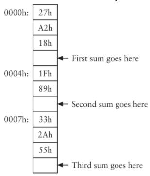
This is how I'll be showing a section of memory in this book. The boxes represent the contents of the memory. Each byte of memory is in a box. The address of that box is at the left. Not every address needs to be indicated because the addresses are sequential and you can always figure out what address applies to a particular box. At the right are some comments about
