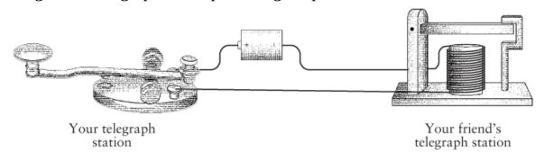
As we discovered, you don't need two wires connecting the two telegraph stations. One wire will suffice if the earth provides the other half of the circuit.
