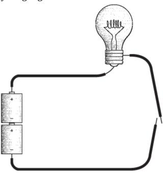
Notice the two loose ends of the wires at the right of the diagram. That's our switch. Assuming that the batteries are good and the bulb isn't burned out, touching these loose ends together will turn on the light.
