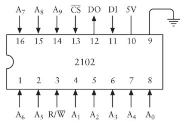
The 2102 is a member of the MOS (metal-oxide semiconductor) family of semiconductors, which is the same technology used for the 8080 and 6800 microprocessors themselves. MOS semiconductors can be easily connected to TTL chips; they generally have a higher density of transistors than TTL but aren't as fast.
