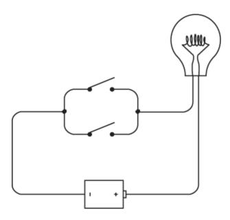
These switches are said to be connected *in parallel*. The difference between this and the preceding connection is that this lightbulb will light if you close the top switch:
