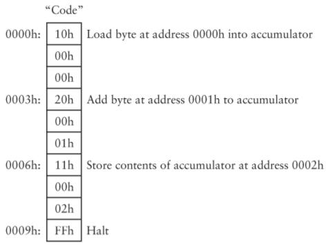
Each of the instruction codes (except *Halt*) is followed by 2 bytes that indicate a 16-bit address in the Data RAM array. These three addresses happen to be 0000h, 0001h, and 0002h, but they could be anything.
