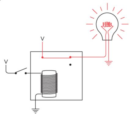
In this case, the lightbulb goes out when you close the switch. A single relay wired in this way is called an *inverter*. An inverter isn't a logic gate
