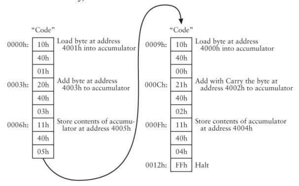
Notice that the 2 low-order bytes located at addresses 4001h and 4003h are added first, with the result stored at address 4005h. The 2 high-order bytes (at addresses 4000h and 4002h) are added with the *Add with Carry* instruction, and the result is stored at address 4004h. And if we were to
