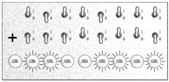
In this diagram, the switches are set to add 183 (or 10110111) and 22 (00010110), producing the result of 205, or 11001101 as shown in the row
