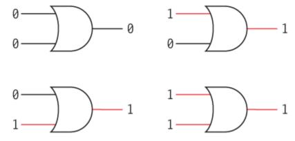
In the same way that we summarized the output of the AND gate, we can summarize the output of the OR gate:
