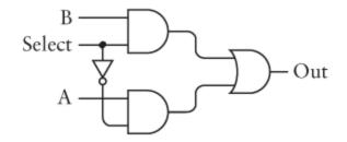
If the Select input is 1, the output of the OR gate is the same as the B input. That's because the output of the top AND gate is the same as the B input, and the output of the bottom AND gate is 0. Similarly, if the Select input is 0, the output is the same as the A input. This is summed up in the following function table:
