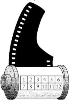
You'll see a checkerboard-like grid of silver and black squares that I've numbered 1 through 12 in the diagram. This is called *DX-encoding*. These 12 squares are actually 12 bits. A silver square means a 1 bit and a black square means a 0 bit. Square 1 and square 7 are always silver (1).
