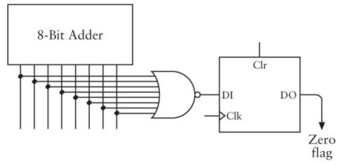
The output of that 8-bit NOR gate is 1 only if all the inputs are 0. Like the Clock input of the Carry latch, the Clock input of the Zero latch latches a value only when an *Add, Subtract, Add with Carry*, or *Subtract with*
