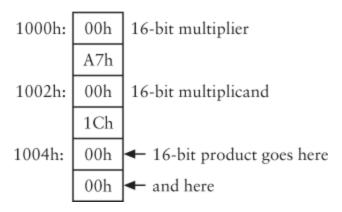
Everyone knows that multiplying A7h and 1Ch (which is 28 in decimal) is the same as 28 additions of A7h. So the 16-bit location at addresses 1004h and 1005h will actually be an accumulated summation. Here's the code for adding A7h to that location once:
