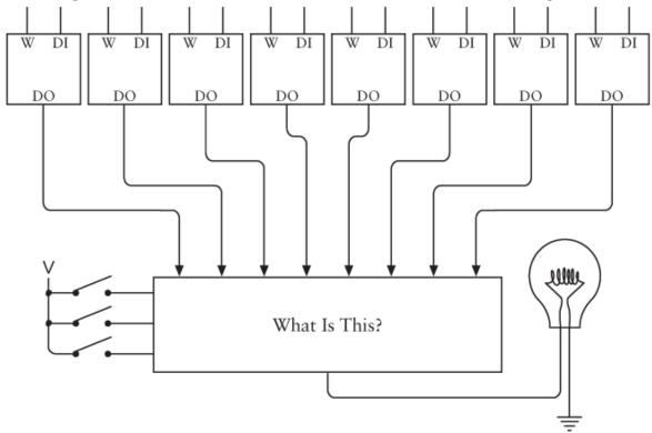
The "something else" is that mysterious box with eight inputs on top and three inputs on the left. By closing and opening the three switches, we can select which of the eight inputs is routed to the output at the bottom of the box. This output lights up the lightbulb.
