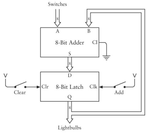
Notice that the switch labeled *Add* now controls the Clock input of the latch.
