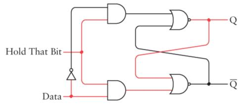
The Q output is now the same as the Data input, and  $\overline{\mathbb{Q}}$  is the opposite. Now Hold That Bit can go back to being 0:
