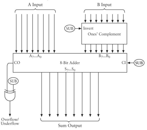
Notice the three signals all labeled *SUB*. This is the Add/Subtract switch. This signal is 0 if an addition is to be performed and 1 if a subtraction is to
