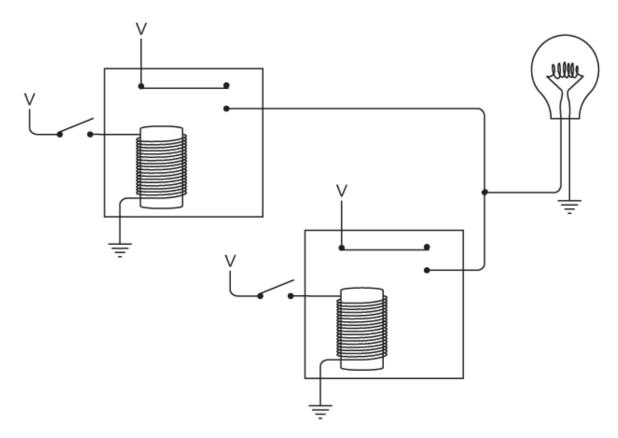
Notice that the outputs of the two relays are connected to each other. This connected output then provides power for the lightbulb. Either one of the two relays is enough to light the bulb. For example, if we close the top switch, the bulb lights up. The bulb is getting power from the left relay.
