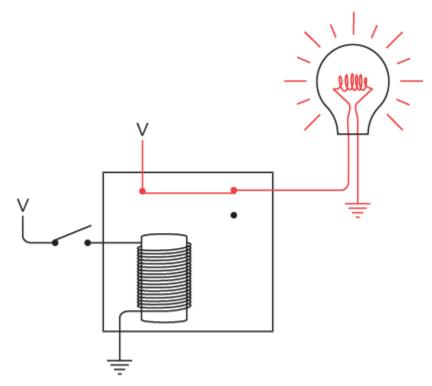
And when the input switch is closed, the bulb goes out:
