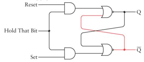
Recall that the output of an AND gate is 1 only if both inputs are 1. In this diagram, the Q output is 0 and the  $\overline{\mathbb{Q}}$  output is 1.
