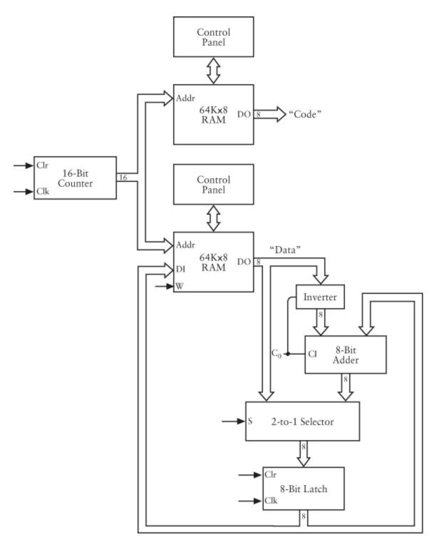
Now suppose we wish to add 56h and 2Ah together and then subtract 38h from the sum. You can do it with the following codes and data stored in the two RAM arrays:
