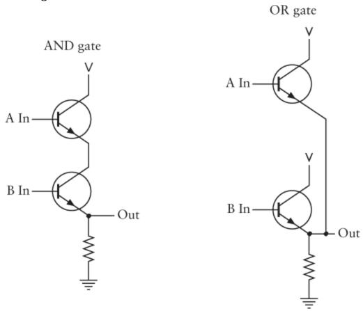
So everything we learned about constructing logic gates and other components from relays is valid for transistors. Relays, tubes, and transistors were all initially developed primarily for purposes of amplification but can be connected in similar ways to make logic gates out of which computers can be built. The first transistor computers were built in 1956, and within a few years tubes had been abandoned for the design of new computers.
