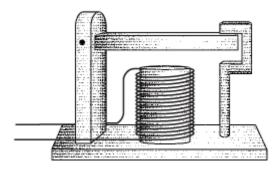
When the telegraph key was pressed, the electromagnet in the sounder pulled the movable bar down and it made a "click" noise. When the key was released, the bar sprang back to its normal position, making a "clack" noise. A fast "click-clack" was a dot; a slower "click...clack" was a dash.
