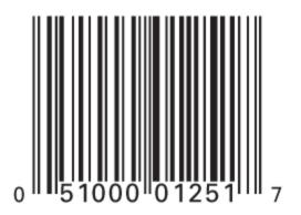
We're tempted to try to visually interpret the UPC in terms of thin bars and black bars, narrow gaps and wide gaps, and indeed, that's one way to look at it. The black bars in the UPC can have four different widths, with the thicker bars being two, three, and four times the width of the thinnest bar. Similarly, the wider gaps between the bars are two, three, and four times the width of the thinnest gap.
