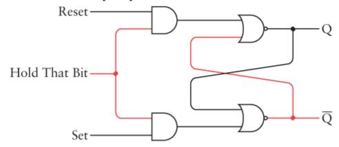
It behaves like a normal R-S flip-flop because now the output of the upper AND gate is the same as the Reset signal, and the output of the lower AND gate is the same as the Set signal.
