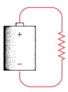
The squiggly line is recognizable to electrical engineers as the symbol for a resistor. Here it means that the circuit has a resistance that is neither very low nor very high.
