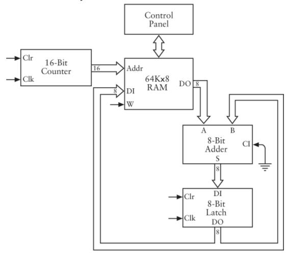
I've eliminated some other parts of the automated adder in this diagram as well, specifically the oscillator and the Clear switch. I removed them because it's no longer at all obvious where the Clear and Clock inputs to the counter and the latch will come from. Moreover, now that we've made use of the RAM data inputs, we need a way to control the RAM Write signal.
