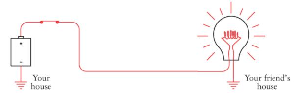
The electrons come out of the earth at your friend's house, go through the lightbulb and wire, the switch at your house, and then go into the positive terminal of the battery. Electrons from the negative terminal of the battery go into the earth.
