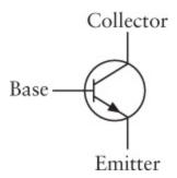
A small voltage on the base can control a much larger voltage passing from the collector to the emitter. If there's no voltage on the base, it effectively turns off the transistor.
