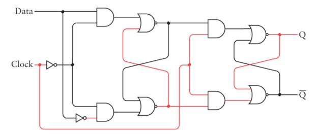
The Q and  $\overline{\mathbb{Q}}$  outputs can change only at the instant that the Clock input changes from 0 to 1.
