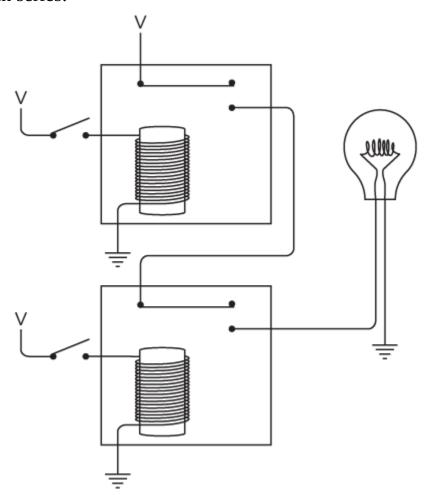
The output of the top relay supplies a voltage to the second relay. As you can see, when both switches are open, the lightbulb isn't lit. We can try closing the top switch:
