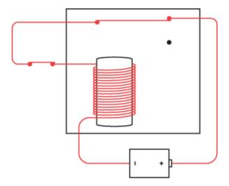
which, of course, completes the circuit again. What happens is this: As long as the switch is closed, the metal contact goes back and forth—alternately closing the circuit and opening it—most likely making a sound. If the contact makes a rasping sound, it's a buzzer. If you attach a hammer to it and provide a metal gong, you'll have the makings of an electric bell.
