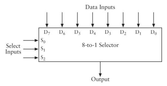
The 8-to-1 Selector has eight Data inputs (shown at the top) and three Select inputs (shown at the left). The Select inputs choose which of the Data inputs appears at the Output. For example, if the Select inputs are 000, the Output is the same as  $D_0$ . If the Select inputs are 111, the Output is the same as  $D_7$ . If the Select inputs are 101, the Output is the same as  $D_5$ . Here's the logic table:
