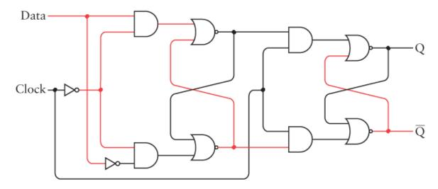
This changes the first flip-flop stage because the inverted Clock input is 1. But the second stage remains unchanged because the uninverted Clock input is 0. Now change the Clock input to 1:
