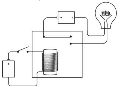
Notice that the switch at the left is open and the lightbulb is off. When you close the switch, the battery at the left causes current to flow through the many turns of wire around the iron bar. The iron bar becomes magnetic and pulls down a flexible metal contact that connects the circuit to turn on the lightbulb:
