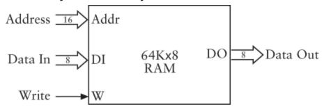
Why 64 KB? Why not 32 KB or 128 KB? *Because 65,536 is a nice round number*. It's 2<sup>16</sup>. This RAM array has a 16-bit address. In other words, the address is 2 bytes exactly. In hexadecimal, the address ranges from 0000h through FFFFh.
