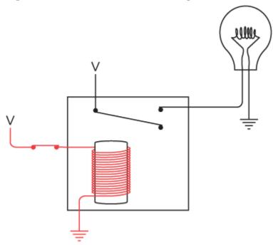
Using the terminology of switches, this type of relay is called a *double-throw* relay. It has two outputs that are electrically opposite—when one has
