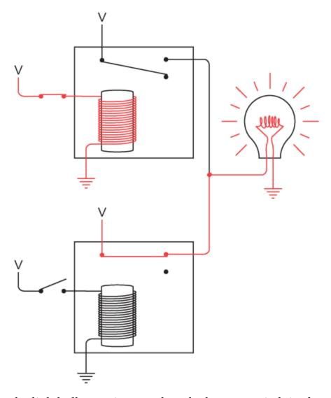
Similarly, the lightbulb remains on when the bottom switch is closed:
