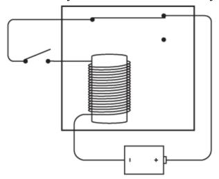
If this looks a little odd to you, you're not imagining things. We haven't seen a relay wired quite like this yet. Usually a relay is wired so that the input is separate from the output. Here it's all one big circle. If you close the switch, a circuit is completed:
