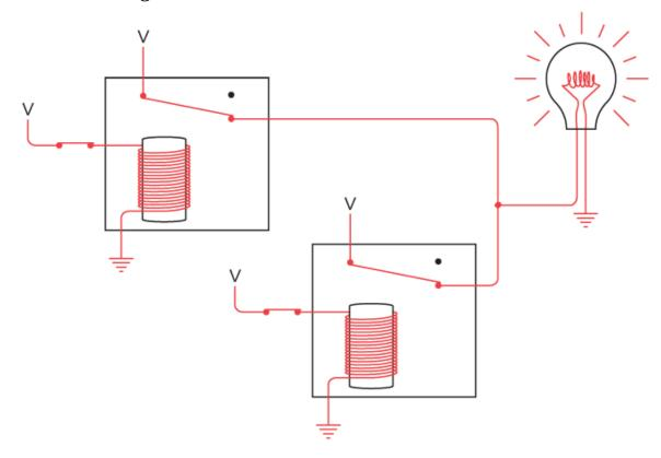
What we have here is a situation in which the bulb lights up if the top switch *or* the bottom switch is closed. The key word here is *or*, so this is called the *OR gate*. Electrical engineers use a symbol for the OR gate that looks like this:
