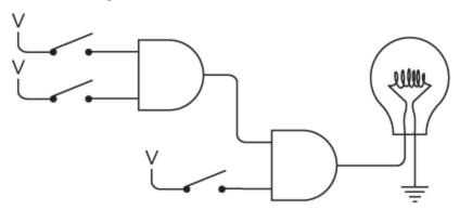
This bulb will light up only if all three switches are closed. Only if the top two switches are closed will the output of the first AND gate trigger the first relay in the second AND gate. The bottom switch triggers the second relay in the second AND gate.
