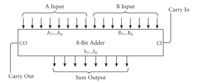
This is a common way to label the separate bits of a multibit number. The bits  $A_0$ ,  $B_0$ , and  $S_0$  are the *least-significant*, or rightmost, bits. The bits  $A_7$ ,  $B_7$ , and  $S_7$  are the *most-significant*, or leftmost, bits. For example, here's how these subscripted letters would apply to the binary number 0110-1001:
