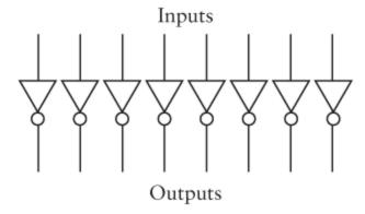
The problem with this circuit is that it *always* inverts the bits that enter into it. We're trying to create a machine that does both addition and subtraction, so the circuitry needs to invert the bits only if a subtraction is being performed. A better circuit looks like this:
