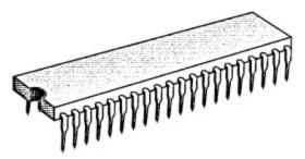
Of course, what you see is just the packaging. The actual wafer of silicon inside is much smaller—in the case of the early 8-bit microprocessors, the silicon is less than ¼ inch square. The packaging protects the silicon chip and also provides access to all of the chip's input and output points through the pins. The diagram on the following page shows the function of the 40 pins of the 8080.
