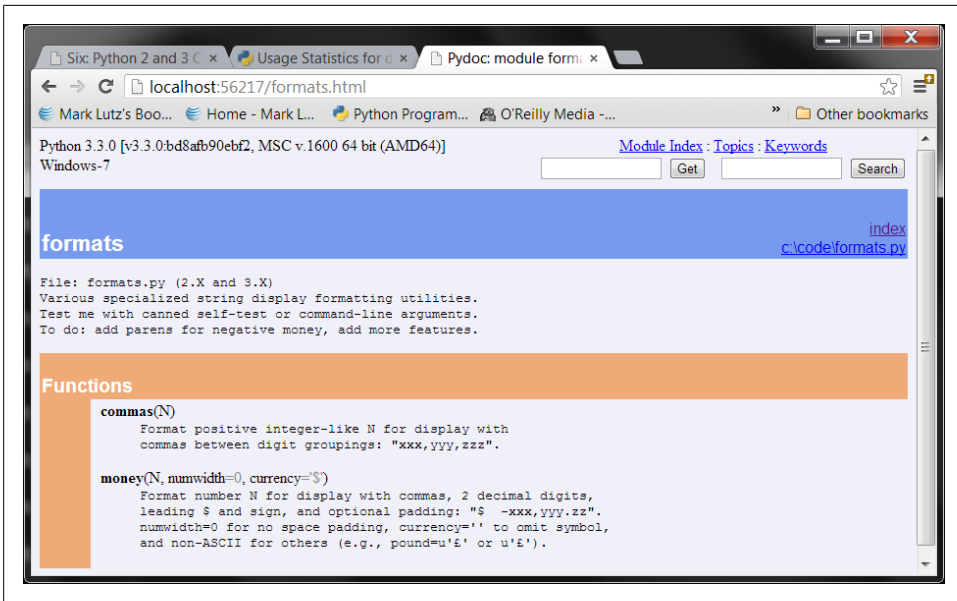
Figure 25-2. PyDoc’s view of formats.py , obtained by running a “ py -3 -m pydoc -b ” command line in 3.2 and later and clicking on the file’s index entry (see Chapter 15)
