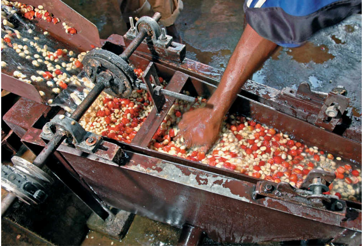
At a coffee washing station in Butare, a worker keeps the coffee cherries moving as the depulping machine separates the seeds from the fruit flesh.
