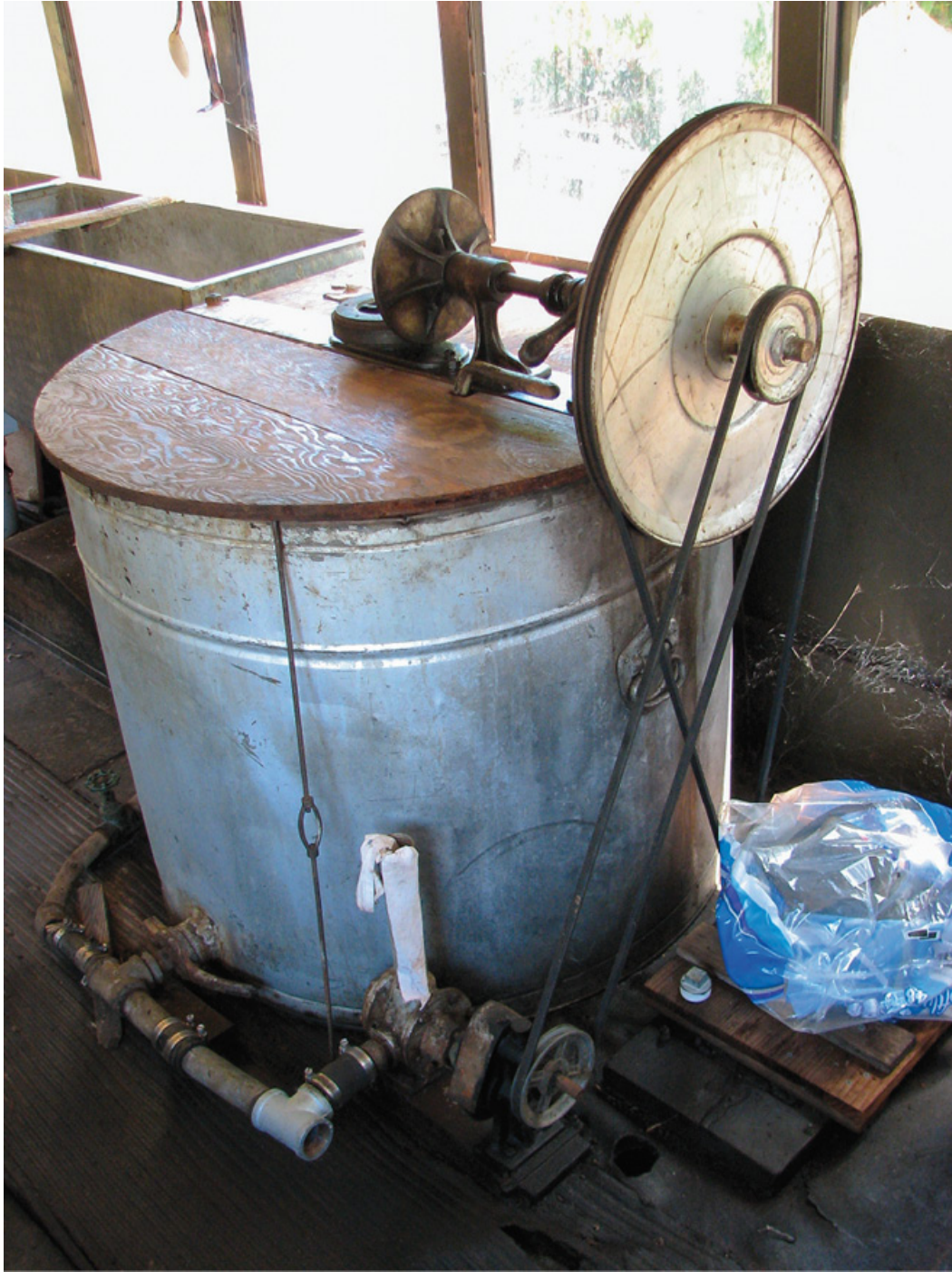
The honey spinner, or extractor, used to spin honey out of uncapped honeycomb using centrifugal force. The pulleys were powered by a motor Grandpa cribbed from a lawn mower (hidden under the plastic). (Photo by Jenn Jackson)
