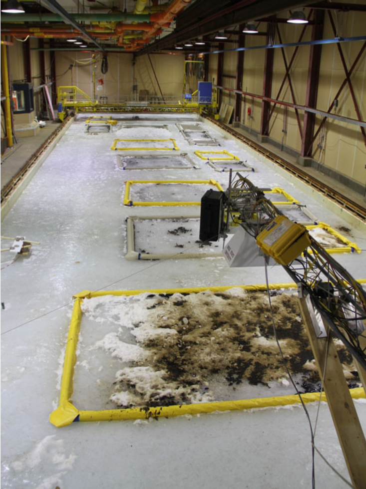
Fig. 2 CRREL facility with oiled containment hoops and boom mounted with surface sensors (source: CRREL (Cold Regions Research and Engineering Laboratory))
