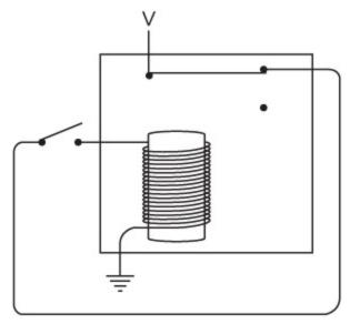
You might recognize in this diagram the inverter from Chapter 11. The circuit can be drawn more simply this way:
