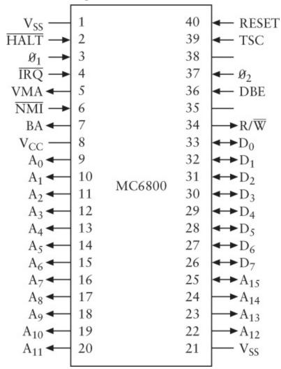
The  $V_{SS}$  indicates Ground, and  $V_{CC}$  is 5 volts. Like the 8080, the 6800 has 16 output Address signals and 8 Data signals used for both input and output.
