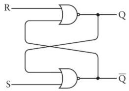
The output that we used for the lightbulb is traditionally called Q. In addition, there's a second output called  $\overline{\mathbb{Q}}$  (pronounced Q bar) that's the opposite of Q. If Q is 0, then  $\overline{\mathbb{Q}}$  is 1, and vice versa. The two inputs are called S for set and
