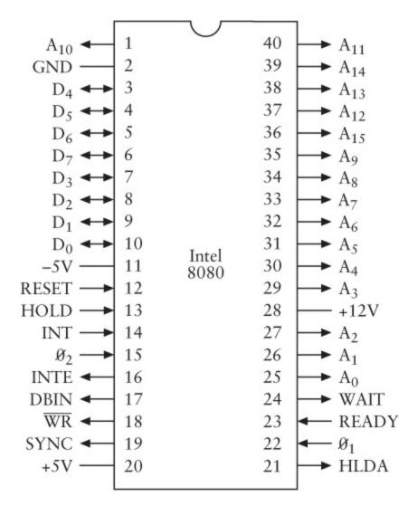
Every electrical or electronic device that we've built in this book has required some kind of electrical power supply. One of the 8080's quirks is that it requires three power supply voltages. Pin 20 must be connected to a 5-volt power supply, pin 11 to a –5-volt power supply, and pin 28 to a 12-volt power supply. You connect pin 2 to ground. (In 1976, Intel released the 8085 chip, which simplified these power requirements.)
