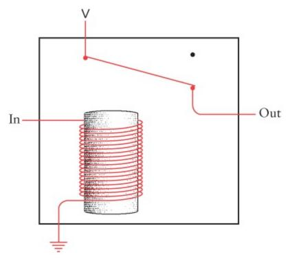
So a telegraph key, a relay, and a sounder are connected more or less like
