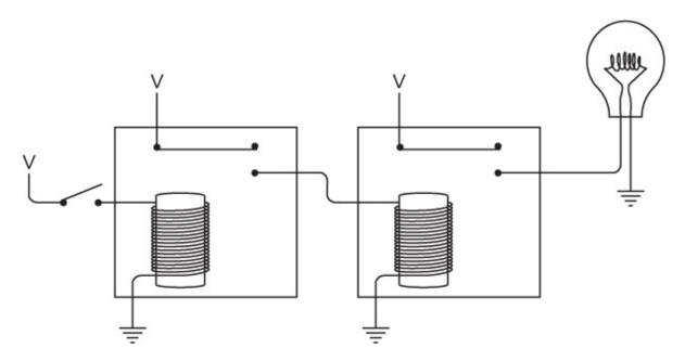
When you turn the switch on, the first relay is triggered, which then provides a voltage to the second relay. The second relay is triggered and the light goes on:
