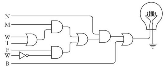
The symbols down the left side of the circuit diagram are in the same order as they appear in the expression. These signals come from the switches wired with inverters and the 2-line-to-4-line decoder. Notice the use of the inverter for the (1 - W) part of the expression.
