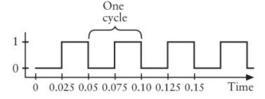
The frequency of the oscillator is 1 divided by the period. In this example, if the period of the oscillator is 0.05 second, the frequency of the oscillator is 1  $\div$  0.05, or 20 cycles per second. Twenty times per second, the output of the oscillator changes and changes back.
