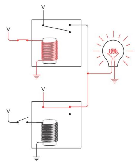
Similarly, the lightbulb remains on when the bottom switch is closed:
