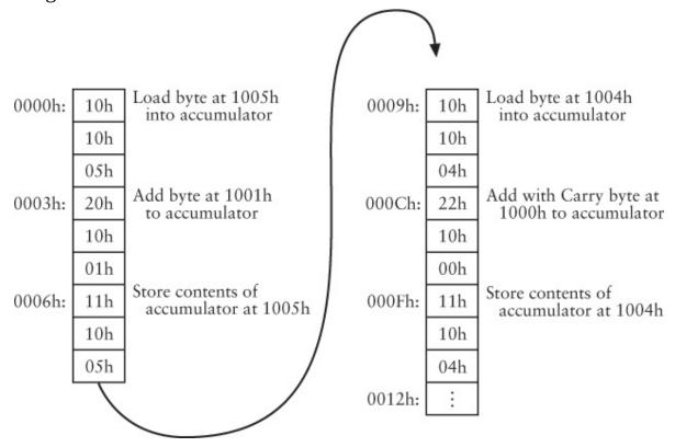
At the completion of these six instructions, the 16-bit value at memory locations 1004h and 1005h will equal A7h times 1. Therefore, these six instructions have to be repeated 27 more times in order for that 16-bit value to equal A7h times 1Ch. You can achieve this by typing in these six instructions 27 more times beginning at address 0012h. Or you can put a Halt instruction at 0012h and press the Reset button 28 times to get the final
