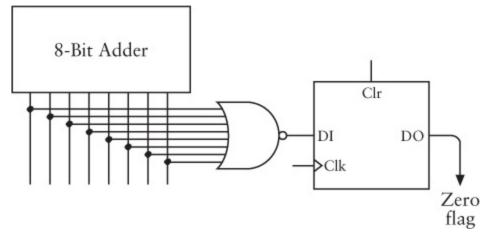
The output of that 8-bit NOR gate is 1 only if all the inputs are 0. Like the Clock input of the Carry latch, the Clock input of the Zero latch latches a value only when an Add, Subtract, Add with Carry, or Subtract with Borrow
