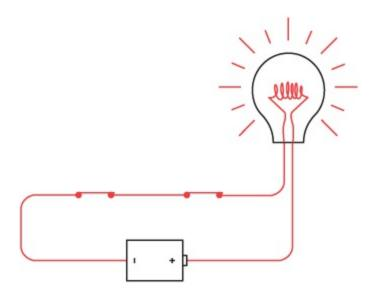
The key word here is and. Both the left switch and the right switch must be closed for the current to flow through the circuit.
