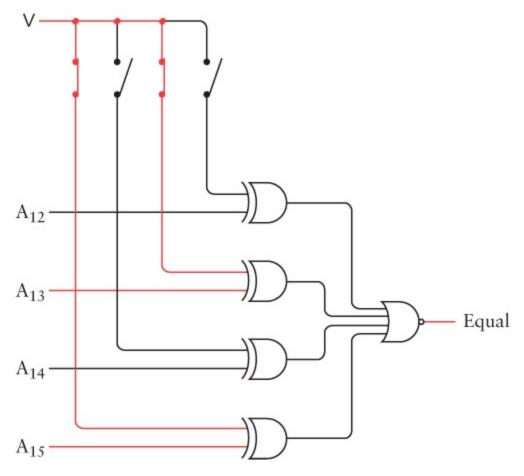
You can then combine that Equal signal with a 2-Line-to-4-Line Decoder to generate  $\overline{\text{CS}}$  signals for each of the four banks of memory:
