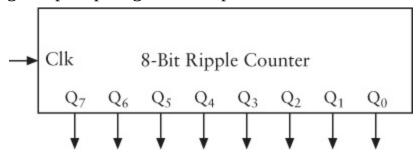
This is called a ripple counter because the output of each flip-flop becomes the Clock input of the next flip-flop. Changes ripple through the stages sequentially, and the flip-flops at the end might be delayed a little in changing. More sophisticated counters are synchronous, in which all the outputs change at the same time.
