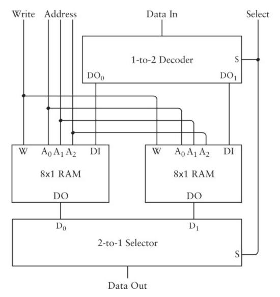
The Select input that goes to both the Decoder and the Selector essentially selects between the two 8 x 1 RAM arrays. It's really a fourth address line. So this is actually a 16 x 1 RAM array:
