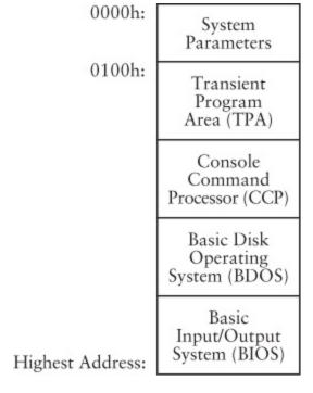
This diagram isn't to scale. The three components of CP/M—the Basic Input/ Output System (BIOS), the Basic Disk Operating System (BDOS), and the Console Command Processor (CCP)—occupy only about 6 KB of memory in total. The Transient Program Area (TPA)—about 58 KB of memory in a 64-KB computer—initially contains nothing.
