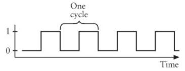
The time required for one cycle is called the period of the oscillator. Let's assume that we're looking at a particular oscillator that has a period of 0.05 second. We can then label the horizontal axis in seconds beginning from some arbitrary time we denote as 0:
