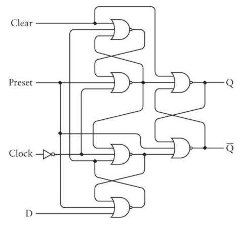
The Preset and Clear inputs override the Clock and Data inputs. Normally these two inputs are 0. When the Preset input is 1, Q becomes 1 and  $\overline{\mathbb{Q}}$
