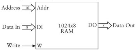
This RAM array stores a total of 8196 bits, organized as 1024 values of eight bits each. There are ten Address inputs because 2<sup>10</sup> equals 1024. There are eight Data inputs and eight Data outputs.
