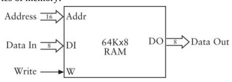
Why 64 KB? Why not 32 KB or 128 KB? Because 65,536 is a nice round number. It's 2<sup>16</sup>. This RAM array has a 16-bit address. In other words, the address is 2 bytes exactly. In hexadecimal, the address ranges from 0000h through FFFFh.
