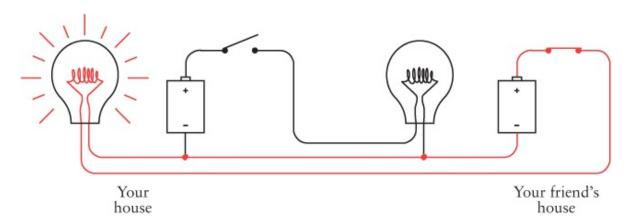
When you and your friend both try to send at the same time, sometimes both switches are open, sometimes one switch is closed but the other is open, and sometimes both switches are depressed. In that case, the flow of electricity in the circuit looks like this:
