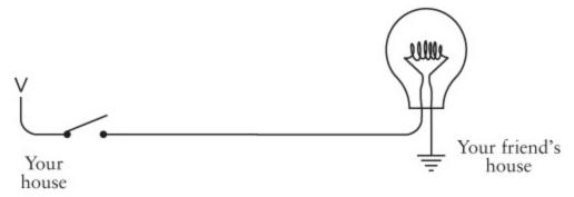
The V stands for voltage, but it could also stand for vacuum. Think of the V as an electron vacuum and think of the ground as an ocean of electrons. The
