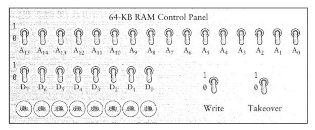
All the switches are shown in their off (0) positions. I've also included a switch labeled Takeover. The purpose of this switch is to let other circuits use the same memory that the control panel is connected to. When the switch is set to 0 (as shown), the rest of the switches on the control panel don't do anything. When the switch is set to 1, however, the control panel has exclusive control over the memory.
