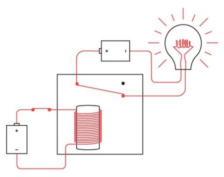
When the electromagnet pulls the metal contact, the relay is said to be triggered. When the switch is turned off, the iron bar stops being magnetic, and the metal contact returns to its normal position.
