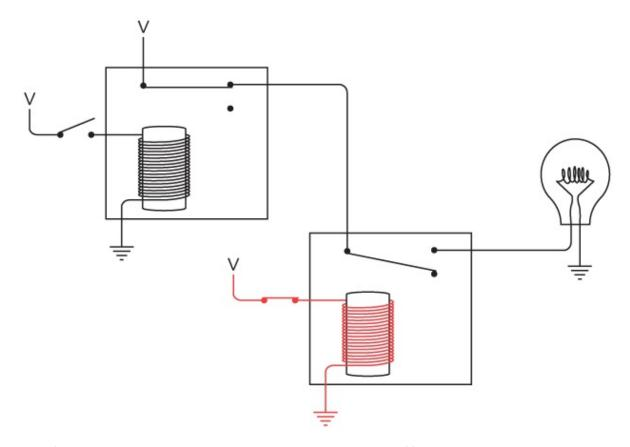
And if both switches are closed, the lightbulb is off:
