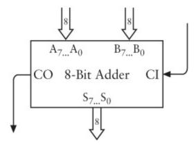
Normally (ignoring what we did with subtraction in the last chapter), the eight A inputs and eight B inputs are connected to switches, the CI (Carry In) input is connected to ground, and the eight S (Sum) outputs and CO (Carry Out) are connected to lightbulbs.
