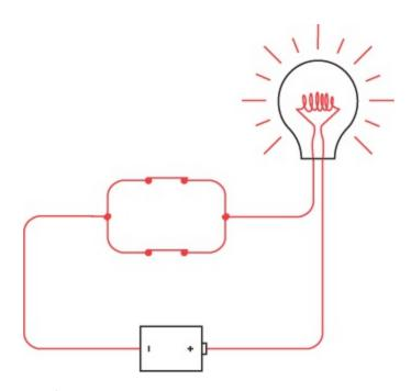
The lightbulb lights if the top switch or the bottom switch is closed. The key word here is or.
