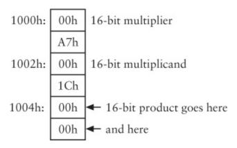
Everyone knows that multiplying A7h and 1Ch (which is 28 in decimal) is the same as 28 additions of A7h. So the 16-bit location at addresses 1004h and 1005h will actually be an accumulated summation. Here's the code for adding A7h to that location once:
