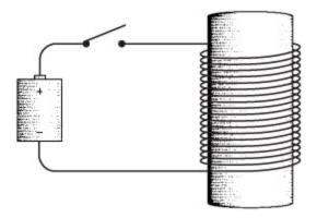
The electromagnet is the foundation of the telegraph. Turning the switch on and off at one end causes the electromagnet to do something at the other end.
