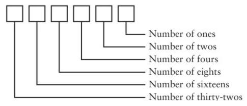
So anytime we have a binary number composed of a 1 followed by all zeros, that number is a power of two. The power is the same as the number of zeros in the binary number. Here's our expanded table of the powers of two demonstrating this rule:
