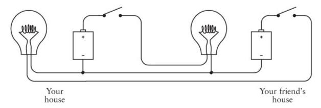
Notice that the negative terminals of the two batteries are now connected. The two circular circuits (battery to switch to bulb to battery) still operate independently, even though they're now joined like Siamese twins.
