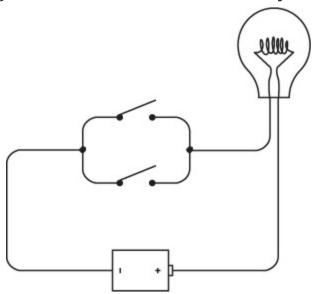
These switches are said to be connected in parallel. The difference between
