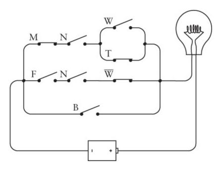
Although the M, T, and NOT W switches are closed, we don't have a complete circuit to light up the lightbulb. Next the salesperson brought out a neutered white female:
