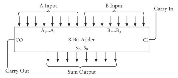
As you probably recall, the inputs A0 through A7 and B0 through B7 were connected to switches that indicated two 8-bit values to be added. The Carry In input was connected to ground. The S0 through S7 outputs were connected to eight lightbulbs that displayed the result of the addition. Because the addition could result in a 9-bit value, the Carry Out output was also connected to a ninth lightbulb.
