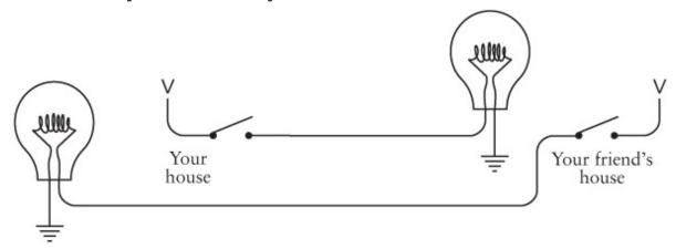
This circuit is functionally the same as the configuration shown previously, in which three wires crossed the fence between the houses.
