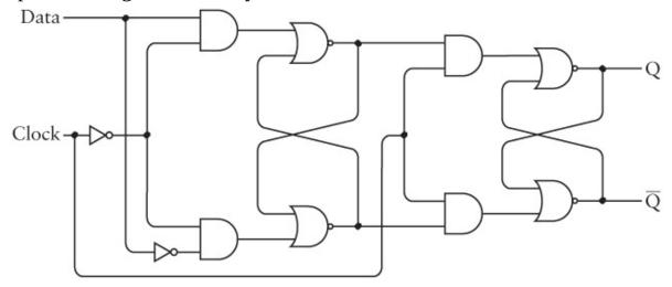
The idea here is that the Clock input controls both the first stage and the second stage. But notice that the clock is inverted in the first stage. This means that the first stage works exactly like a D-type flip-flop except that the Data input is stored when the Clock is 0. The outputs of the second stage are inputs to the first stage, and these are saved when the Clock is 1. The overall result is that the Data input is saved when the Clock changes from 0 to 1.
