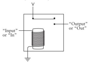
If a current is flowing through the input (for example, if a switch connects the input to V), the electromagnet is triggered and the output has a voltage.
