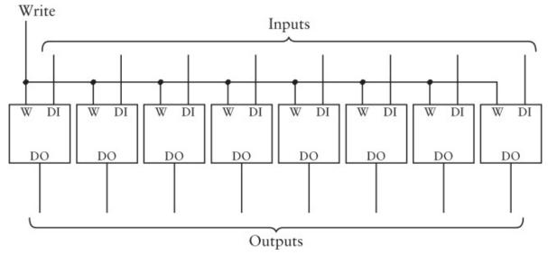
This 8-bit latch has eight inputs and eight outputs. In addition, the latch has a single input named Write that's normally 0. To save an 8-bit value in this latch, make the Write input 1 and then 0 again. This latch can also be drawn as a single box, like so:
