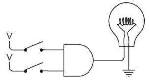
Notice that this symbol for the AND gate not only takes the place of two relays wired in series, but it also implies that the top relay is connected to a voltage, and both relays are connected to ground. Again, the lightbulb lights
