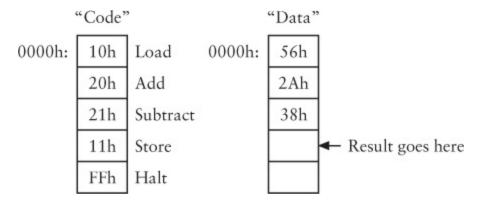
After the Load operation, the accumulator contains the value 56h. After the Add operation, the accumulator contains the sum of 56h and 2Ah, or 80h. The Subtract operation causes the bits of the next value in the Data RAM array (38h) to be inverted. The inverted value C7h is added to 80h with the carry input of the adder set to 1:
