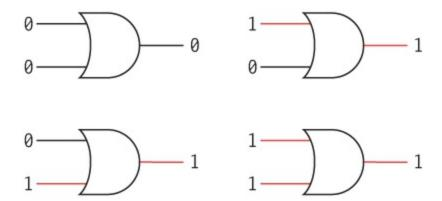
In the same way that we summarized the output of the AND gate, we can summarize the output of the OR gate:
