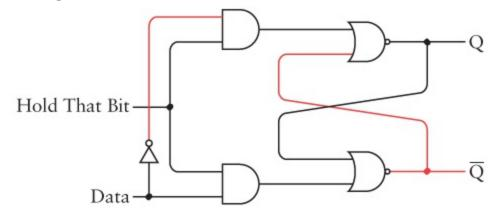
In this case, both inputs are 0 and the output Q is 0 (which means that  $\overline{Q}$  is 1). As long as Hold That Bit is 0, the Data input has no effect on the circuit:
