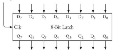
This latch is capable of saving 8 bits at once. The eight inputs on the top are labeled  $D_0$  through  $D_7$ , and the eight outputs on the bottom are labeled  $Q_0$  through  $Q_7$ . The input at the left is the Clock. The Clock signal is normally 0. When the Clock signal is 1, the 8-bit value on the D inputs is transferred to the Q outputs. When the Clock signal goes back to 0, that 8-bit value stays there until the next time the Clock signal is 1.
