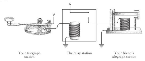
The relay is a remarkable device. It's a switch, surely, but a switch that's turned on and off not by human hands but by a current. You could do amazing things with such devices. You could actually assemble much of a computer with them.
