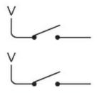
When both switches are open (as shown), they indicate the color white. Here's how to use two inverters and one AND gate to generate a signal I'll call W, which is a voltage (1) if you select a white cat and not a voltage (0) if not:
