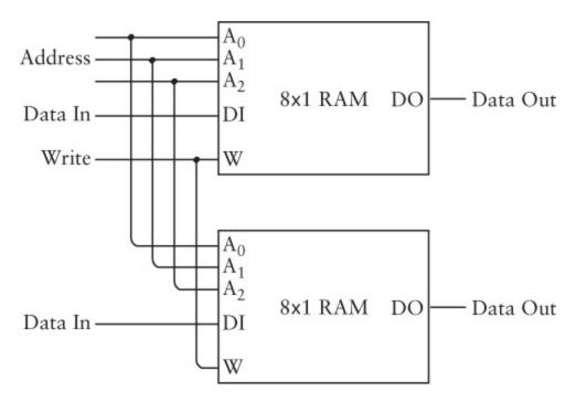
The Address and Write inputs of the two 8 x 1 RAM arrays are connected, so the result is an 8 x 2 RAM array:
