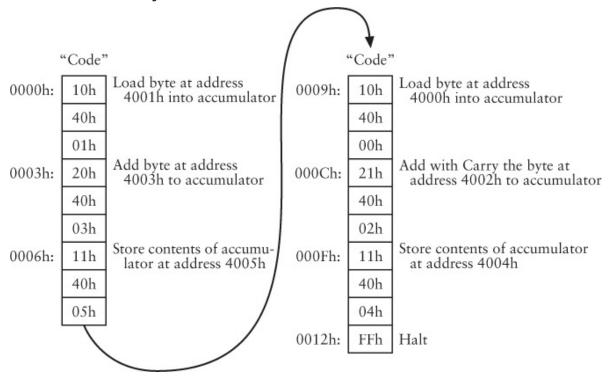
Notice that the 2 low-order bytes located at addresses 4001h and 4003h are added first, with the result stored at address 4005h. The 2 high-order bytes (at addresses 4000h and 4002h) are added with the Add with Carry instruction, and the result is stored at address 4004h. And if we were to remove the Halt instruction and add more instructions to the Code memory, a sub-sequent calculation could later make use of the original numbers and the sum of them
