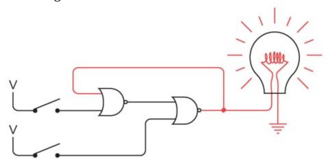
Now this is odd, wouldn't you say? Both switches are open—the same as in the first drawing—yet now the lightbulb is on. This situation is certainly different from anything we've seen before. Usually the output of a circuit is dependent solely upon the inputs. That doesn't seem to be the case here. Moreover, at this point you can close and open that upper switch and the light remains lit. That switch has no further effect on the circuit because the output of the left NOR gate remains 0.
