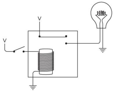
When the switch is closed, the bulb lights up.
