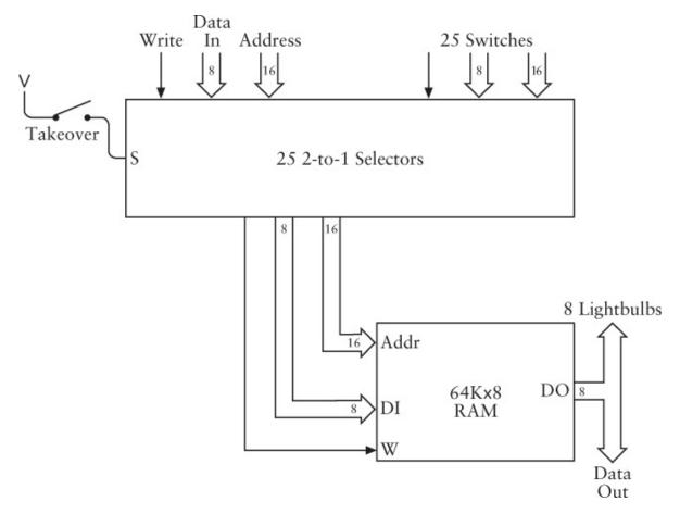
When the Takeover switch is open (as shown), the Address, Data input, and Write inputs to the 64K x 8 RAM array come from external signals shown at the top left of the 2-to-1 Selectors. When the Takeover switch is closed, the Address, Data input, and Write signals to the RAM array come from the switches on the control panel. In either case, the Data Out signals from the RAM array go to the eight lightbulbs and possibly someplace else.
