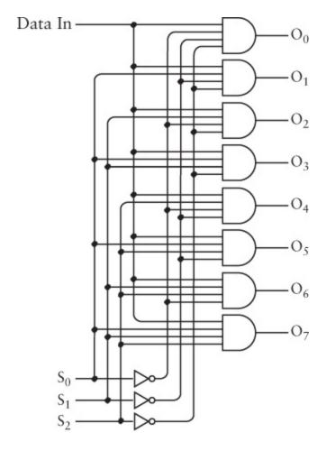
Again, notice that the inputs to the sixth AND gate from the top include  $S_0$ ,  $\overline{S}_1$ ,  $S_2$ . No other AND gate has these three inputs. So if the Select inputs are 101, then all the other AND gates will have an output of 0. The sixth AND gate from the top will possibly have an output of 0 if the Data Input is 0 or an output of 1 if the Data Input is 1. Here's the complete logic table:
