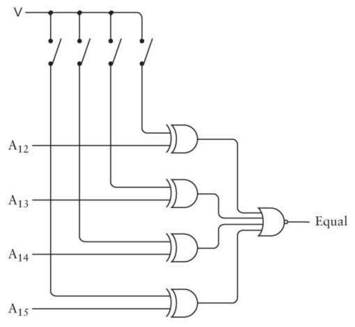
As you'll recall, the output of an XOR gate is 1 if either of the two inputs is 1 but not both. Another way to think of this is that the output of an XOR gate is 0 if the two inputs are the same—either both 0 or both 1.
