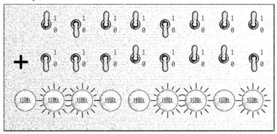
In this diagram, the switches are set to add 183 (or 10110111) and 22 (00010110), producing the result of 205, or 11001101 as shown in the row of lightbulbs.
