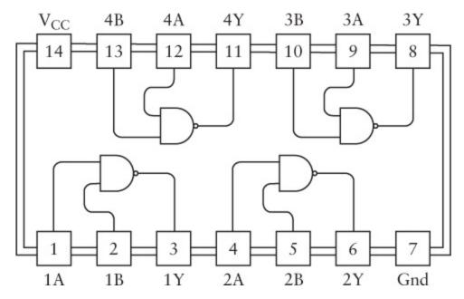
This diagram is a top view of the chip (pins on the bottom) with the little indentation (shown on page 250) at the left.
