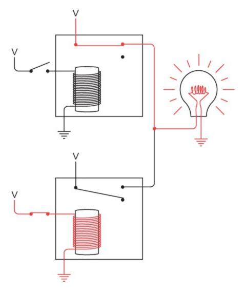
Only when both switches are closed does the lightbulb go off:
