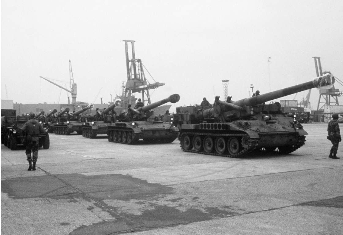
M110 203mm self-propelled Howitzers are staged in a parking area at the port of Antwerp, September 1984. The M110 was capable of firing the W79 Mod 0 shell, a tactical nuclear artillery projectile with an enhanced radiation mode (a “neutron bomb”) that could be switched on or off.
