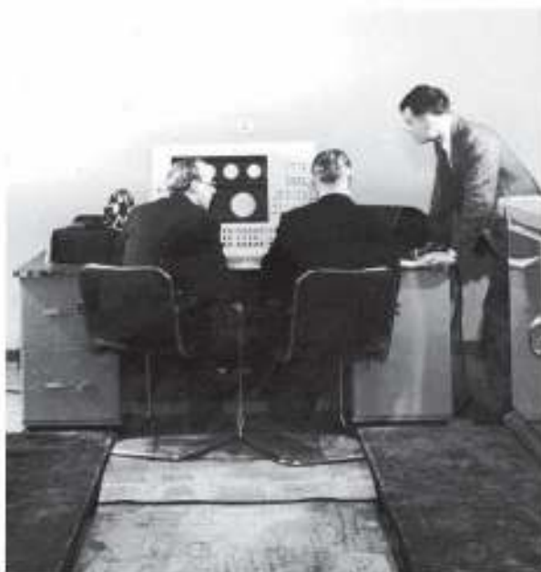
Above: The prototype Manchester computer. The six racks shown are essentially those of the 'baby machine' which ran its first program in June 1948; by June 1949 when this photograph was taken, the machine had roughly doubled in size.
